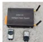
A beautifully-made wireless receiver / GSM dialler in a sturdy metal-clad enclosure. The advantage offered by the wireless GSM unit is that sensors and triggering devices do not need to be hardwired, allowing you to locate the dialler in a more convenient and secure location. It requires a 12V DC supply, which can be derived from the mains using the adaptor provided with the unit, or from a leisure battery if no mains supply is available.
