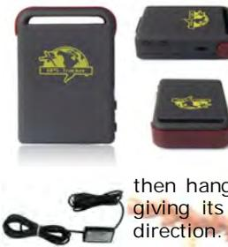
A remarkable little GPS tracking unit that will report its position, speed and direction from anywhere in the world to an accuracy of a few metres. It can be slipped into the pocket of a child or elderly relative, or fixed to an item of machinery (such as a car, tractor or quad-bike). It has an internal rechargeable battery that lasts about 48 hours, and can be connected to a vehicle's 12V supply for continual use. To track it, the user simply calls the number of the sim card,
