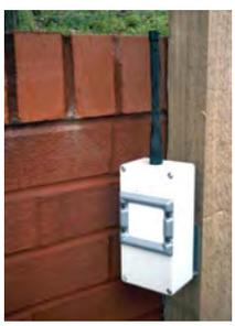
Below is a typical simple application, in which PIR sensors and wireless CCTV cameras are used to protect the two farm entrances. All sensors are completely wireless and self-contained, so can be installed in moments and moved as required with the minimum of fuss. Cameras require mains power, but are otherwise wireless.
